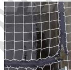
To fit a zip to the net simply use steel hog rings to staple the fabric edging of the zip to the netting, using one staple per mesh square on each side of the net.
